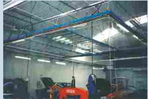
can dissipate and light can come in without increasing the total noise level. The sound absorbing cabin therefore is not a completely closed system, but ensures a 100 percent efficiency with regard to the required and specified insulating value. The installation is very easy in an own sectional system and can be done by the user himself. Windows, escape doors, entrance doors or gates are available in different sizes and can be easily fitted into the cabin.
