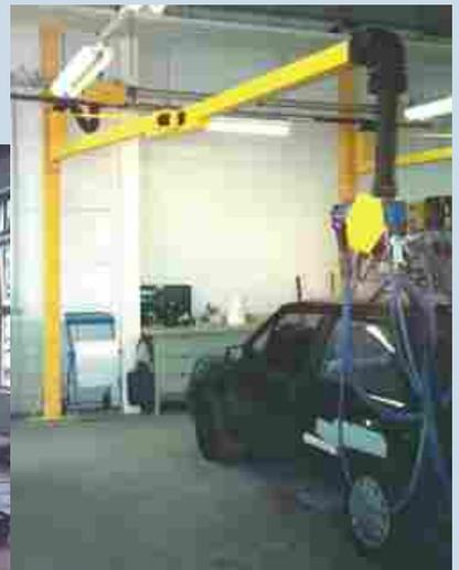
In this case, solid particles, which are heavier than air have to be sucked off instead of gases which expand. A complete suction can only be guaranteed with high air velocities and a high vacuum. This can be realized with hoses small diameters and powerful turbines. AFA is manufacturing stationary compact units and central systems but also mobile suction units for floor cleaning (swarfs suction) which can be compared with a home vacuum cleaner.
