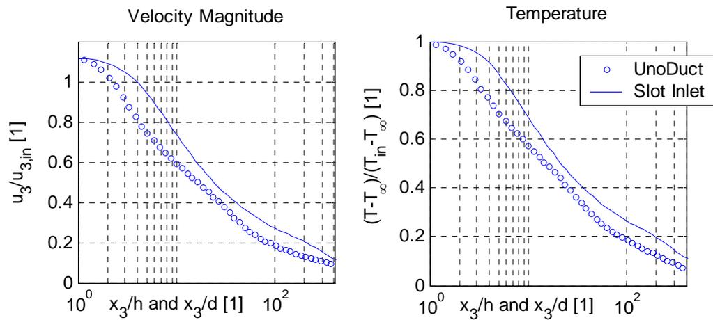
**Figure 7: averaged velocity and temperature on the mean jet centerline**
