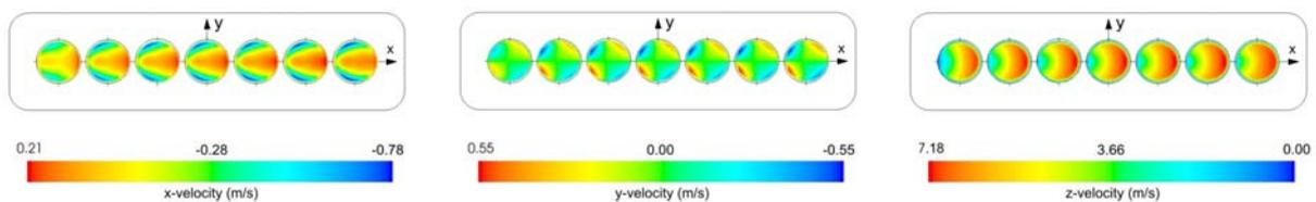
**Figure 2: Contour plot of the double swirl - Uno-Duct supply system ( $p_{\text{stat}}=20\text{Pa}$ ,  $u_{\text{duct}}=4\text{m/s}$ )**
