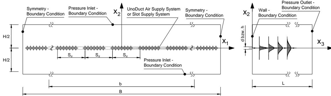
**Figure 3: Boundary conditions of the simulation models**
