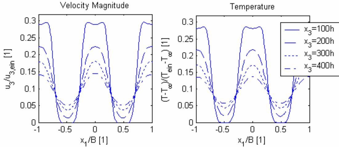
**Figure 5: averaged temperature and temperature – air supply system UnoDuct**
