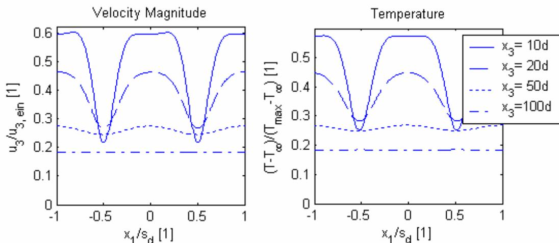
**Figure 4: averaged velocity and temperature – air supply system UnoDuct**
