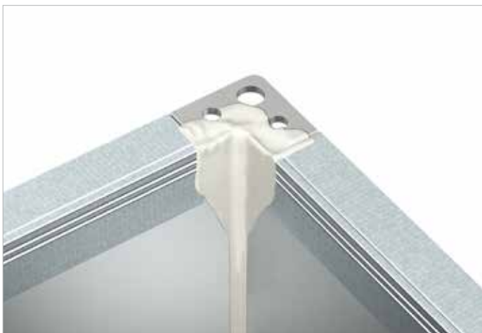
9. Sealing - Apply sealant (e.g. Gebhardt-MAXX, see page 25) at each corner on the inside of the duct. Flanges with BUTYL/GEL don't require any sealing at their longitudinal edge. Keep in mind to seal longitudinal beads as well.
