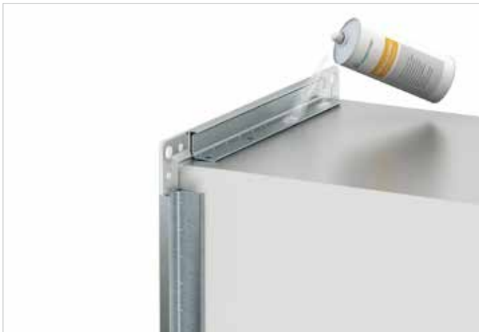
8. Repair spray - Repair spot welding points (depending on flange material) using Zinc-Alu spray or Stainless steel spray (see page 23). This provides corrosion protection and gives the duct a nicer finish.
