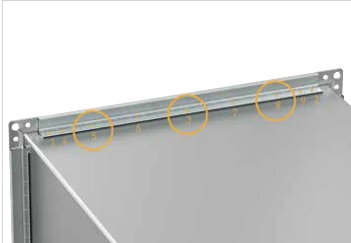
7. Number of spot welding / clinching points - The adhesive force of the inserted Butyl could substitute every second spot welding point, provided that frame assembly is correct.
