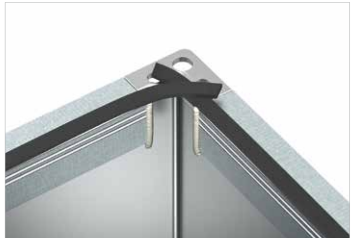
11. Gasket tape - Put on the gasket tape flush to the inner surface of the duct. The gasket tape should overlap in the area of the corners like shown in the figure. Recommended gasket: 20 flange=15x4 mm, 30 flange=20x4 mm, 40 flange=25x4 mm (see page 34)
